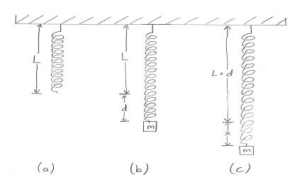
FIGURE 1. (a) A spring in at its natural length, (b) A spring with a weight of mass m attached, (c) A spring with a weight of mass m attached and displaced by a length x
