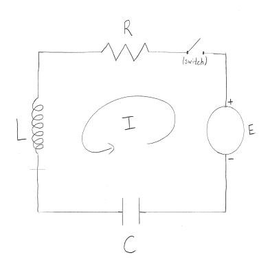
FIGURE 2. A simple RLC circuit. L is the induction coil, R is the resistor, C is capacitor, and E is a battery or generator.
